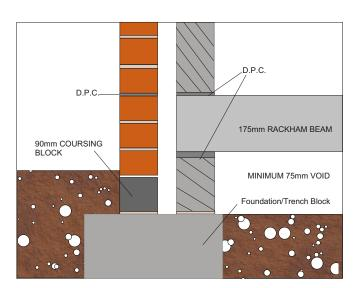
Adequate ventilation should be provided to the underfloor void using one Rackham Ventilator per 3.0 metres of external wall/
